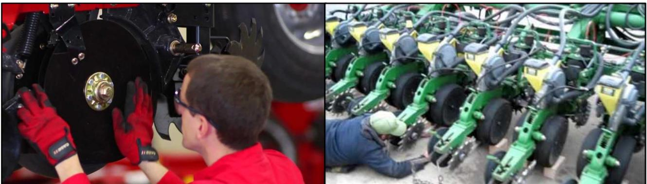
JD opening disks that are worn down to 14.75" from 15" should be replaced. Depth should be preliminarily set in the shop using blocks of the same thickness as the desired depth of planting, by placing them under the gauge wheels and adjusting depth as necessary.
